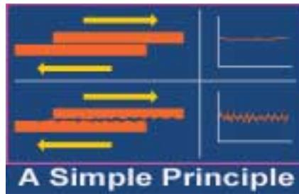
**FIGURE 2**—Rough surfaces produce vibrations.
